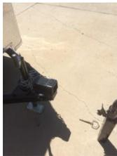
As with anything involving cash, security is of paramount concern. The Removable Hitch option allows you to easily remove the hitch and place it inside the ATMtrailer or in the towing vehicle. Without the hitch the ATMtrailer cannot be moved.
