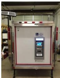
The Solar Maintenance Charger is a 30 Watt solar charger operates to maintain battery charge in the SmartPower system. It can add as much as 30% life to the charge and this can be very helpful when the event lasts longer than most. The solar panel is very impressive when installed on the ATMtrailer and will help attract attention to your ATMtrailer.
